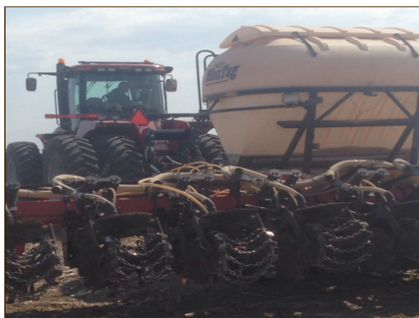
Photo 4. Kuhn Krause gladiator strip-till unit with a Montag fertilizer box used in the on-farm trial.
