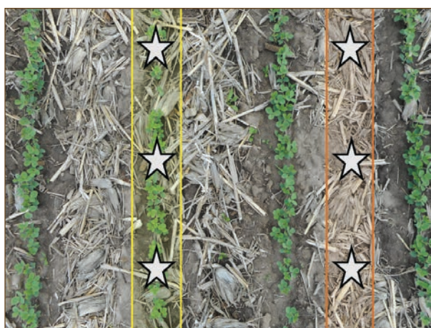
Photo 3. In every plot, three penetrometer measurements were collected in the in-row (I) location and three in the between-row (B) location.
