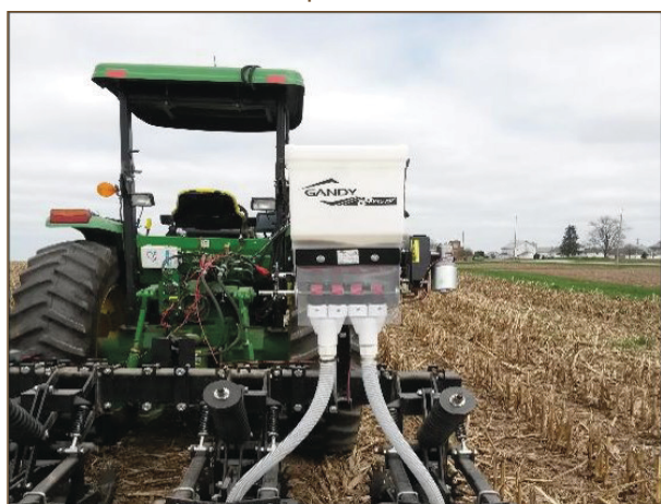
Photo 2. Remlinger strip-till unit with Gandy fertilizer box used in the small plot trial.
